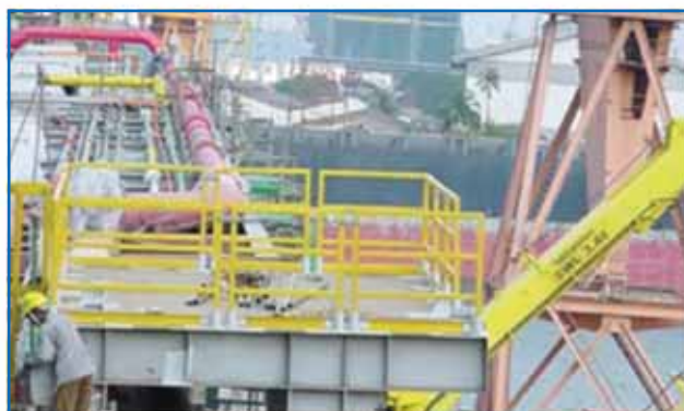
FRP Grating & Handrails For FPSO (Brazil)
